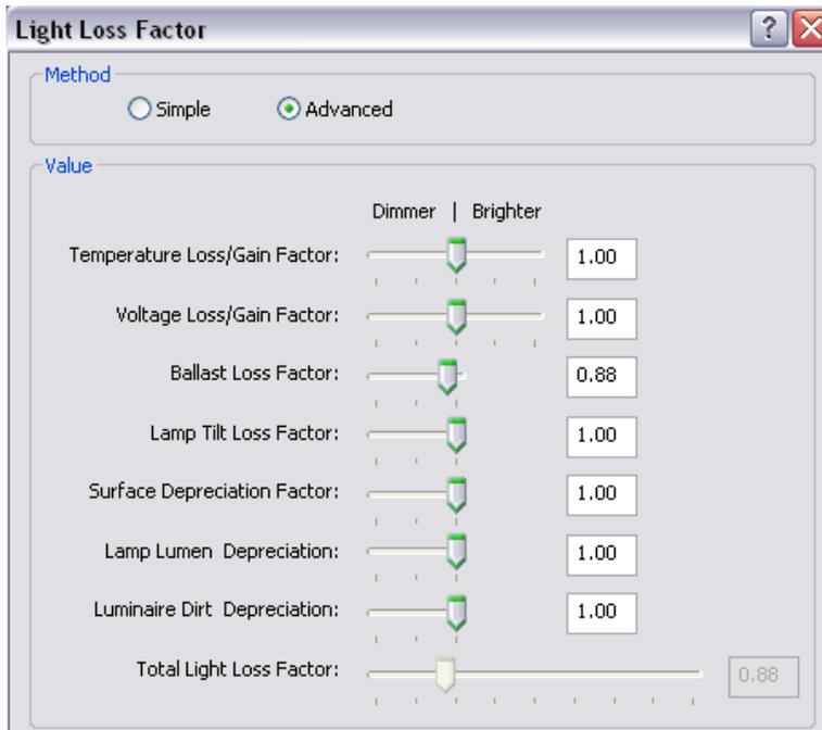
Settings used to calculate Light Loss Factor
