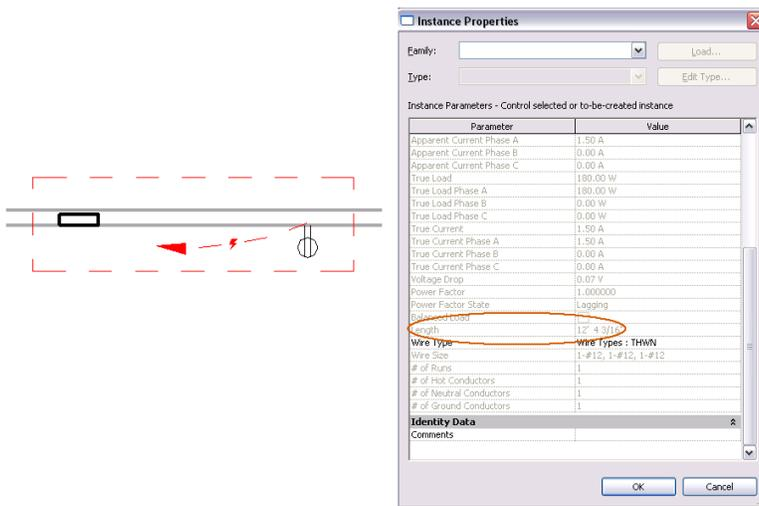
The distance between the receptacle and the panel along the X axis is 10'. However, the panel and the receptacle are at different elevations. The panel is at 4' 0" and the receptacle is at 1' 6", a difference of 2' 6" along the Z axis.
