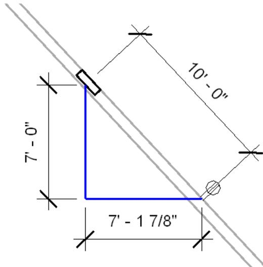
The length is along the X, Y, Z axes is 7' 0" + 7' 1 7/8" + 2' 6" = 16' 7 7/8" and the computed length shown in the circuit properties is 16' 6 13/256".
