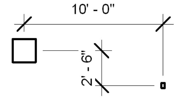
The sum of distances along the X, Y, and Z axes is 12' 6", very close to the 12' 5 9/16" shown for length in the circuit properties. The small difference can be accounted for as the distance to the connector within the components and the measurements that were done to the center of each component.
